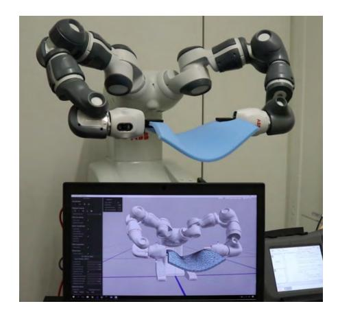
2), to autonomously understand how to grasp, pick up, and dynamically place the soft parcel on a conveyer belt in a prescribed configuration.
