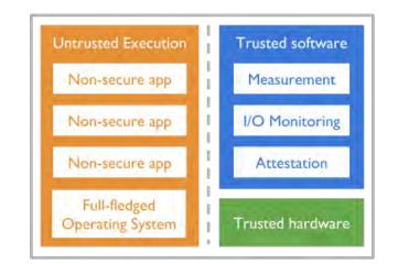
foundation on which trust in the entire device can be established. An example of this are the Security Extensions of Arm's embedded architectures, which provide a hardware-isolated environment in which trusted software (e.g., a verified micro-kernel) can be run to secure core functionalities such as security updates, sensitive cryptographic operations, and software measurement primitives which can be used to verify the rest of the software running on the device.
